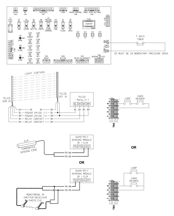
ELR, MONITORING IR, LIGHT CURTAIN, N/O TYPE IR, CARD READER AND LOOP DETECTOR
