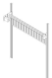
Rolling grille installed on tube supports is as shown. Other products are similar. Angle clips are omitted for clarity. Details are available upon request.
