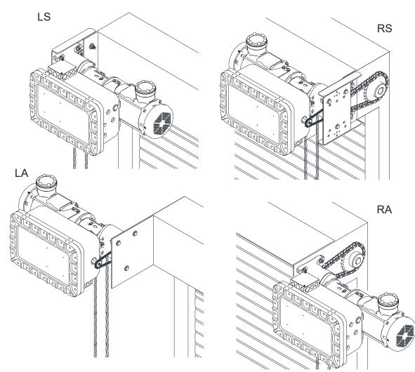
Installation positions for larger horsepower units are similar to as shown above.
