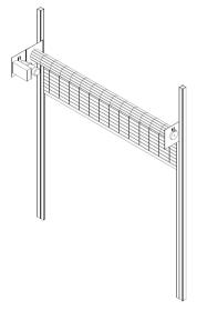
Rolling grille installed on tube supports is as shown. Other products are similar. Angle clips are omitted for clarity. Details are available upon request.
